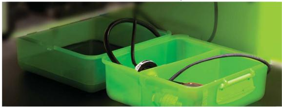
Effectively restore clogged nozzles on XJET & X2 print heads with the Head Recovery System from Inkcups Now! This automatic flushing system utilizes pump technology to continuously flow Nozzle Restore through the print head in order to loosen and remove hardened debris. Simply connect the hose to the desired print head, reposition the container to catch the falling liquid and plug it in! The unit will do all the hard work and you can walk away.
