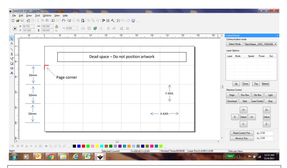
When positioning the artwork, add 7mm to the X-axis coordinate in order to compensate for the table rail. Add 50mm to the Y-axis to compensate for dead space.
